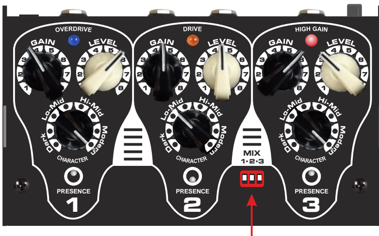
Three sections activated by micro switches
